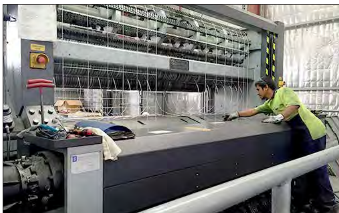
Manufacture of rural mesh at Frauenfelder Gates' Albury factory
