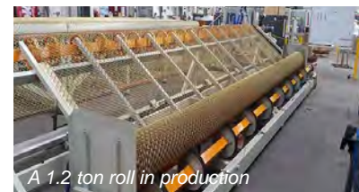
Line wire integrated through the selvedge M-Lokk edge
