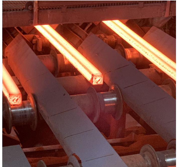
Steel billets being cast at InfraBuild's Sydney Steel Mill
