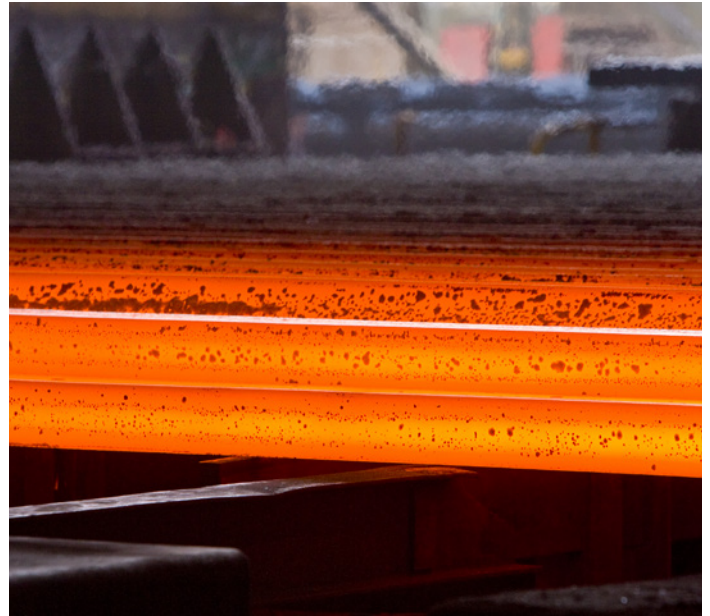
Steel billets being cast at InfraBuild's Sydney Steel Mill
