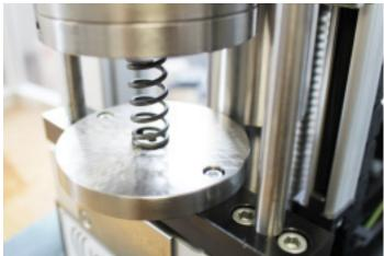
because when a compression spring is deflected, it achieves its linear deflection by twisting the wire.
