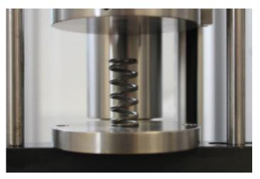
Although more complicated and costly, the benefits in general far outweigh the negatives regarding prestressing. Prestressing not only stabilises the dimensions of the spring, leading to a more predictable product during operation, but also allows the spring to work to higher stresses. Working under higher stresses, springs are more optimised, making them significantly lighter and can save on material costs.
